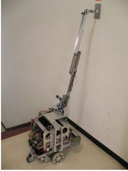
**Figure 9:** Pushing a light switch.
