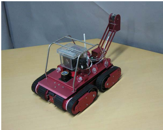
Fig. 20. Prototype robot of mass production version. The robot has a large carrying handle and the shield cover for the inspection camera is made small.
