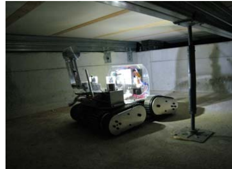
Fig. 14. Under floor environment lightened by LED mounted on the robot.
