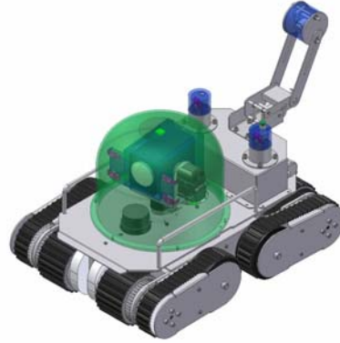
Fig. 6. Design of the inspection robot. It has two main crawlers and four sub-crawlers. Two cameras, a SOKUIKI sensor and a lighting device are mounted on the robot.
