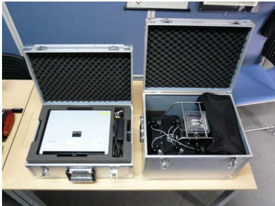
Fig. 21. Carrying cases for operational easiness (left: operational PC, right: robot).
