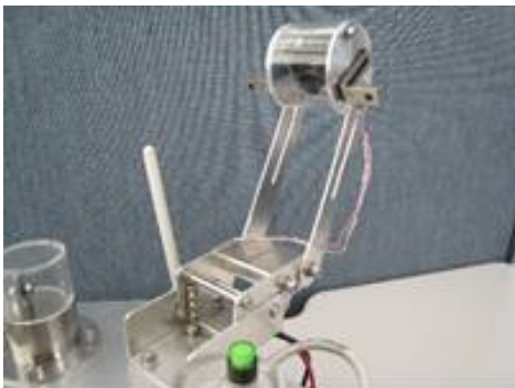
Fig. 9. Bird's-eye camera for robot control.
