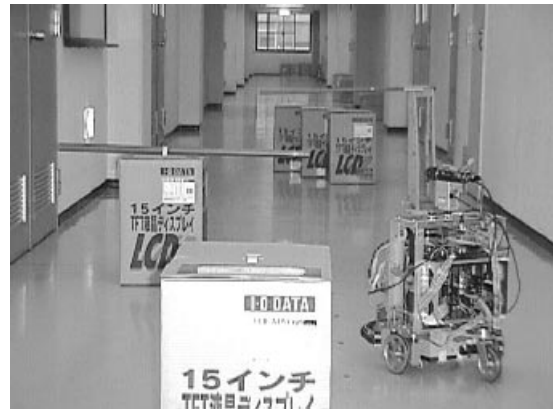
Figure 15: Experimental environment. Several cardboard boxes and resin pipes are placed in a corridor as obstacles.
