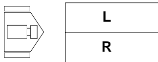
Figure 10: Division of Search Space for collision avoidance. If some object exist in R(L), the robot turns L(R). If some object exists in both sides(R and L), the robot stops and searches a new good passage.
