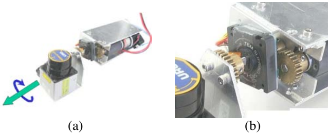
Fig. 6. Rotating device : (a) overall view, (b) slip ring
