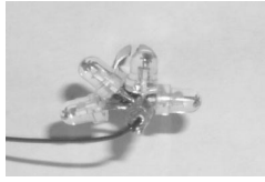
Figure 14: A set of 4 LEDs for direction invariant emission.
