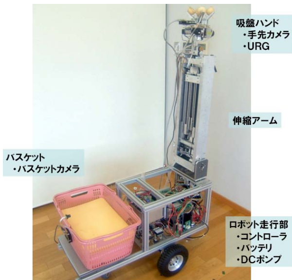
Fig. 4 The integrated shopping robot
