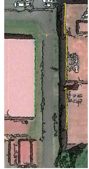
Fig. 8 Result of extracting the highest points for each scan data from from Fig.7
