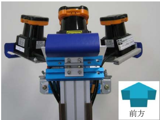
Fig.2 mounted LRFs for Position Correction
