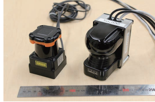
Fig. 1 UTM-30LX(left) and 3D LIDAR (right)
