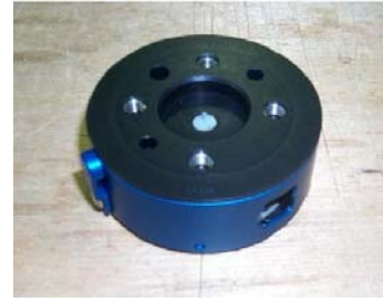
Fig. 4. 6-axis Force sensor.
