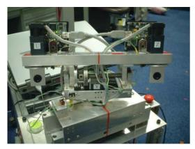
Fig. 6. Stereo camera mounted on the Pan-Tilt device.
