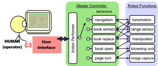
Figure 3: Structure of the software
