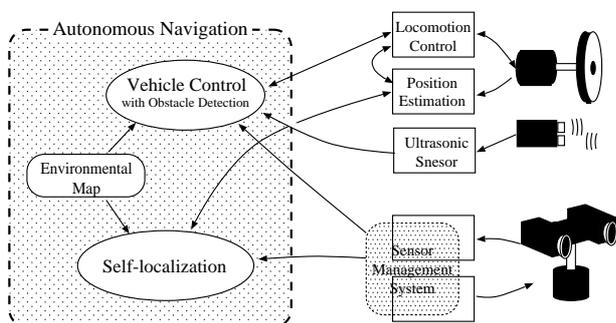
Figure 5: Structure of navigation software.
