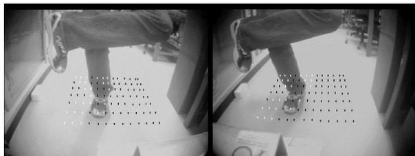
Figure 6: Example of obstacle detection (human leg).
