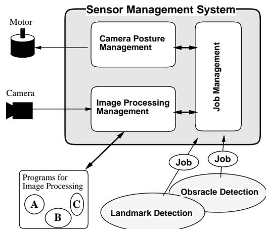
Figure 3: Structure of sensor management system.
