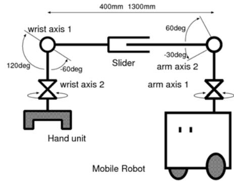
Fig. 3. Hardware Diagram of the Manipulator
