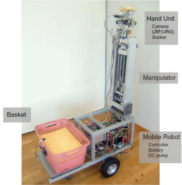
Fig. 5. The Integrated Shopping Robot
