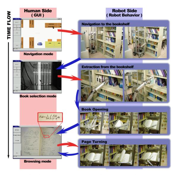
Figure 8: Scenes of an experiment using the all-in-one integrated robot system.
