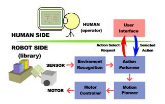
Figure 5: Control system of teleoperation.
