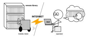
*Figure 1:* Concept of remote book browsing system using a mobile robot.
