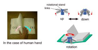
Figure 4: Structure of page turning device.
