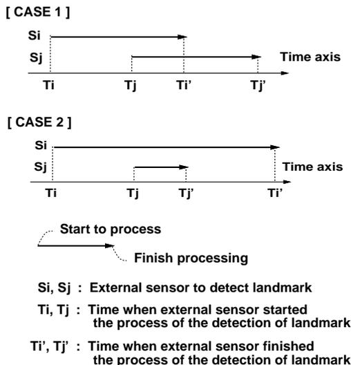
Figure 2: Overlapping on time axis on two landmarks parallel sensing
