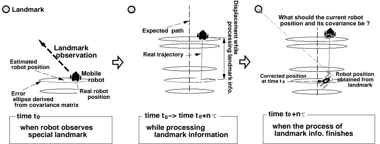
Figure 1: Retroactive positioning data fusion and re-estimation of positional uncertainty at current time
