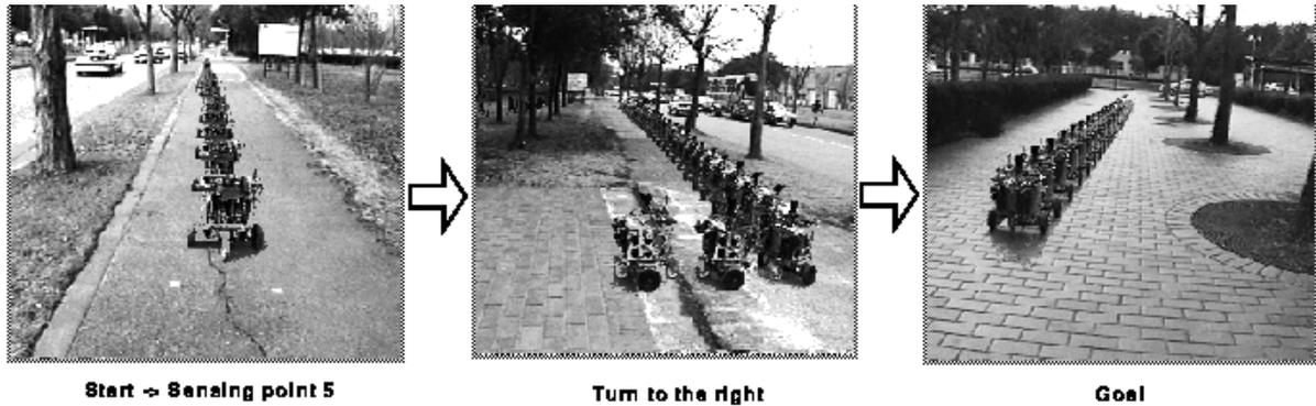
Figure 4: Trajectory of a mobile robot on the experiment of non-stop self-guidance using trees and hedges
