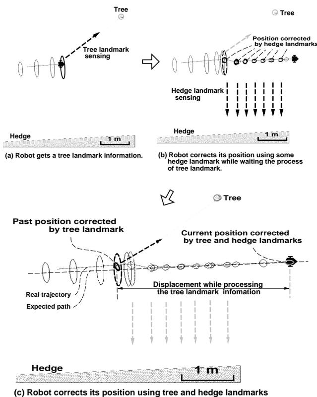
Figure 5: Simulation of retroactive positioning data fusion using tree and hedge landmarks
