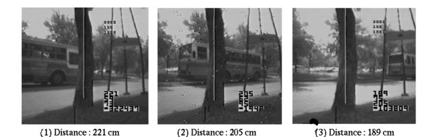
Figure 9: Tree tracking by Tree LmA(Vertical white line indicates the detected tree position in the image)
