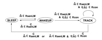
Figure 4: State transition of LmA (RsenLM is validation of the current measurement  $\hat{m}$ . Rcon is geometrical and characteristical condition to judge the same landmark.  $f(\hat{m})$  is the landmark location calculated from  $\hat{m}$ .)
