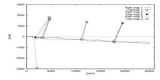
Figure 12: The generated route maps:Path map 1 and Tree map 1 indicate the routmap in the first trial. The points of Tree map indicate the pair of the sensing point and the landmark location.
