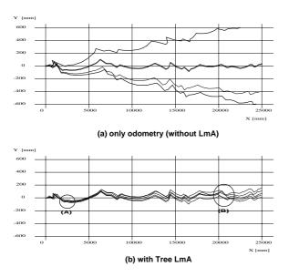
Figure 13: Comparison of the approximated real trajectory in the case of (a)only odometry and (b)odometry and Tree landmarks (Position is corrected by Tree landmarks around (A) and (B).)
