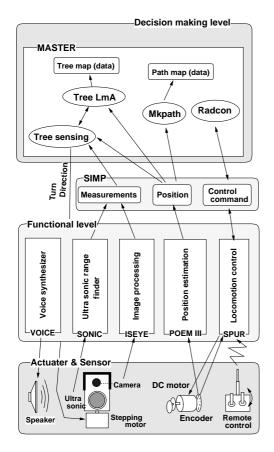
Figure 7: Schematic structure of the YAMABICO NAVI robot controllers (SIMP:State information monitoring panel)
