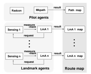
Figure 3: Multiagent programing for route map generation (*Radcon* interprets human operation at the constant interval. *mkpath* records the passing points to Path map at the constant interval. *LmA* is a landmark agent which looks for an assigned landmark and stores the detected landmark to the LmA map. *Sensing* controls a sensing direction and get the sensing results. )
