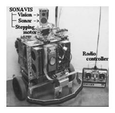
Figure 6: The YAMABICO NAVI robot for the teaching playback navigation robot system(to change the current robot)
