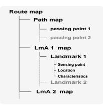
Figure 5: Route map representation separating Path map and each LmA map (Path map:Recording a passing point at the constant interval, LmA map:Recording a sensing point, landmark location and the characteristics )
