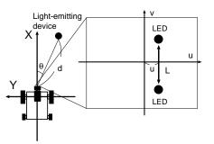
Fig.2 The schema of the image of LEDs obtained from camera mounted on the robot.
