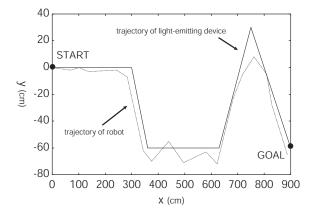
Fig.10 Experimental result of target following using LED.
