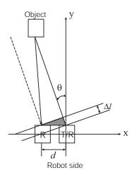
Fig.3 Principles of angle measurement using two ultrasonic receivers.
