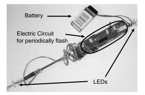
Fig.6 Light-emitting device used in the experiment.
