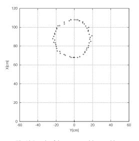
Fig.13 Result of the target position tracking using the ultrasonic transponder.
