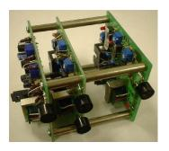
Fig.7 Ultrasonic sensor on the robot.
