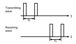
Fig.8 The timing of transmission and reception of the pulses in the double pulse coding.
