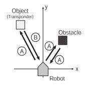
Fig.4 Position detection of a specific object using the ultrasonic transponder.
