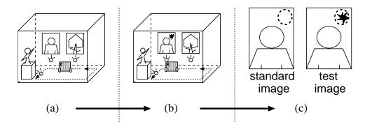
**Fig.**1 Procedures of the indoor monitoring system ((a): Take standard images, (b): Take test images, (c): Compare images)
