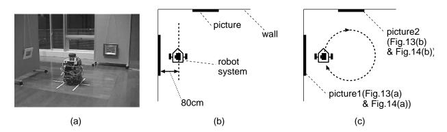
**Fig.**12 Actual experiment of the monitoring system ((a): A view of the experiment, (b): Overhead view of the environment in the experiment, (c): Patrolling route and target pictures for monitoring)
