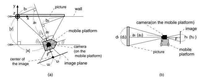
**Fig.**2 Method of calculating the positional relationship of the picture, the robot and camera ((a): Overhead view, (b): Side view)
