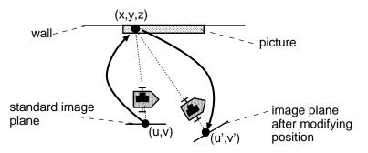
Fig.4 Positional relationship of the robot and a picture used for modifying the image
