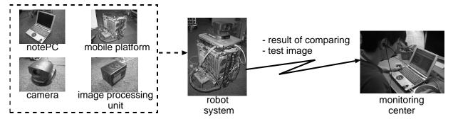
Fig.9 Structure of the robot system
