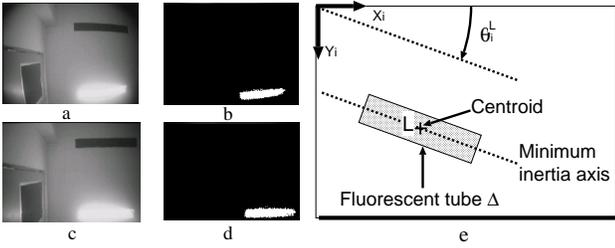
Figure 4. Fluorescent light located on the border of the image. (a),(b) original and binarized images before distortion correction, (c),(d) after distortion correction. (e) Moment-based features of a fluorescent tube.
