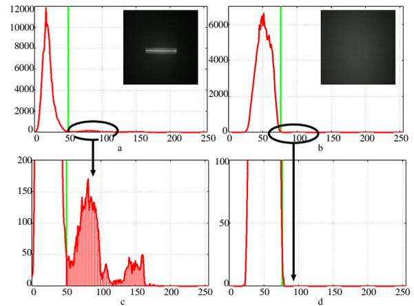
Figure 3. (a) Histogram of a ceiling image containing a light, (b) Histogram of a ceiling image without light. (c) Zoom of (a), (d) zoom of (b). Horizontal axis : grey level (0-255), Vertical axis : pixels number.
