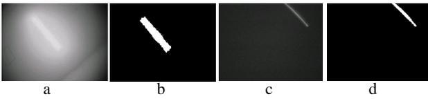
Figure 2. (a),(c) Typical camera images of the ceiling of a corridor containing a fluorescent light. The axis of the camera is perpendicular to the ceiling. (b),(d) Binarized images.
