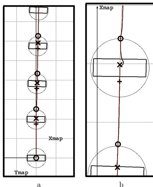
Figure 5. Odometry data of the robot correcting its trajectory using the detection of fluorescent lights in a corridor. (a) Zoom on the first lights, (b) zoom on one light. Rectangles correspond to lights and discs to their detection area. '+': light detected, 'x': *pose* correction, 'o': the robot enters a new segment.
