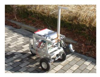
Fig. 1. PWS mobile robot
